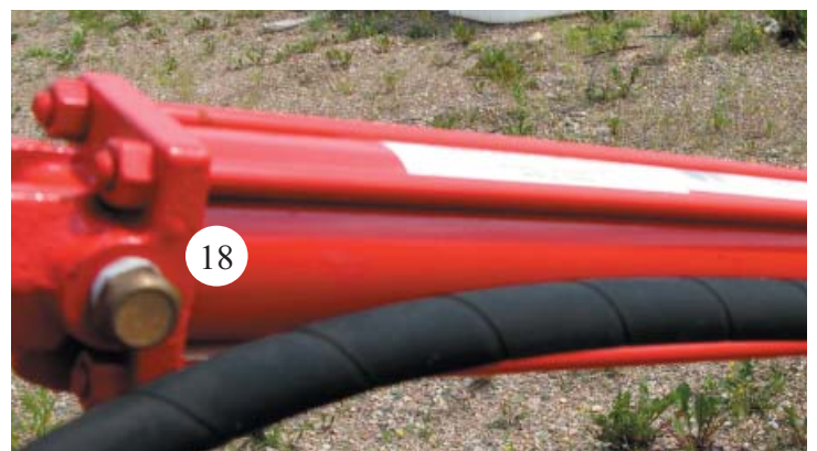
Figure 2.3 - Fitting Assembly of RIGHT Cylinder
