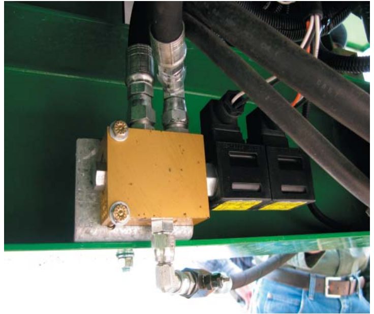
Figure 2.4 -Hydraulic Valve & fittings
