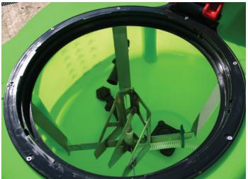
**Mixing:** two agitator jets stir the fluid while the four vertical ribs disrupt the flow increasing the rate of mixing and virtually eliminating the chances of undissolved particles.
