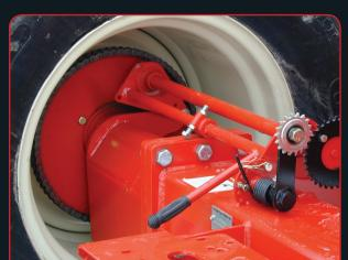
The mechanical ground drive system is "quick detach", has a spring loaded drive chain tensioner and features an adjustment bolt to allow the drive wheel chain and sprocket to remain tight.
