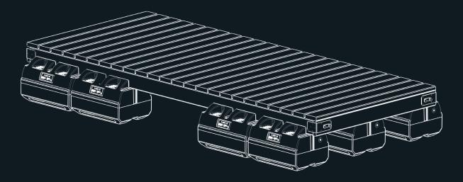
The Polytoon System allows customers to create a dock or platform of any shape and size. The decking is generally made from outdoor wood because the Polytoon systems receiving slots are sized for regular dimensional lumber.
