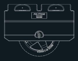
The Polytoon floats are made from high density polyethylene. They are rugged and will not get brittle in cold temperatures. The Polytoons are not only easy to install and low maintenance, they have been designed to incorporate a number of innovative features to ensure endless hours of enjoyment
