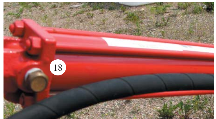
Figure 3.3 - Fitting Assembly of RIGHT Cylinder
