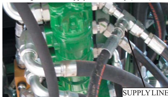
Figure 2.7b -Supply line hook up (D450)
