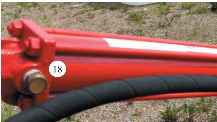
Figure 2.3 - Fitting Assembly of RIGHT Cylinder
