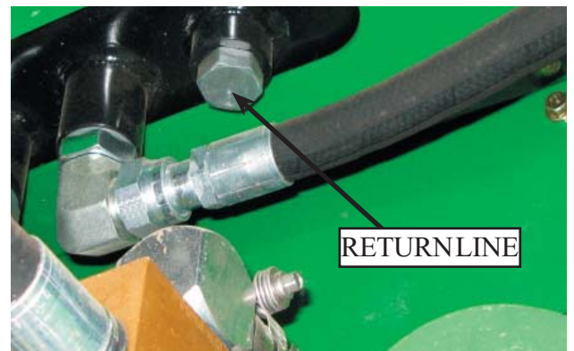
Figure 2.6 - Return line hook up
