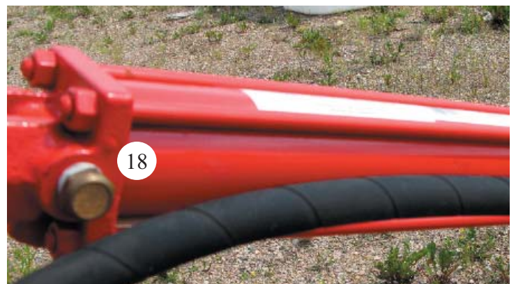
Figure 2.3 - Fitting Assembly of RIGHT Cylinder
