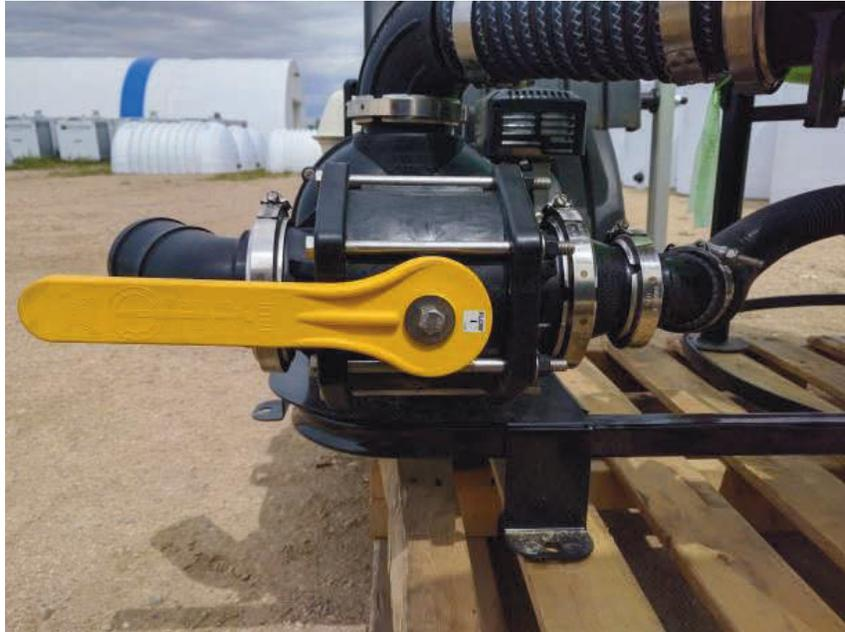
***Figure 5 - Pump Source Selection Tank***
