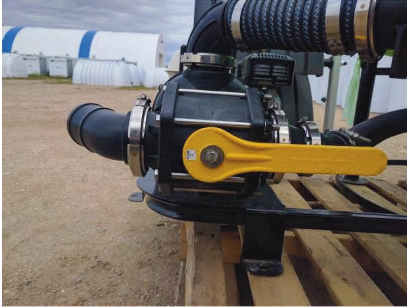
***Figure 7 - Pump Source Selection Chembine***
