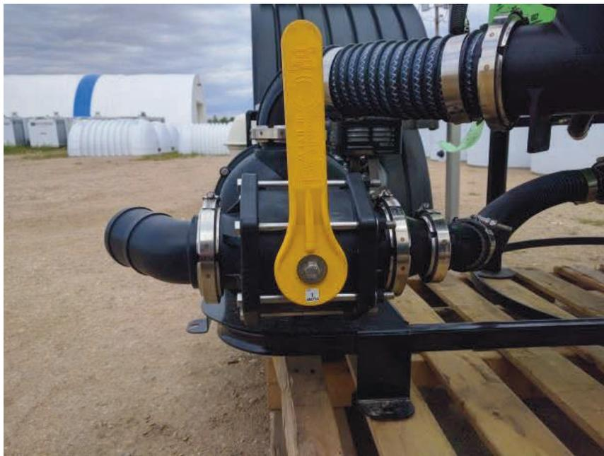
***Figure 6 - Pump Source Selection Off***
