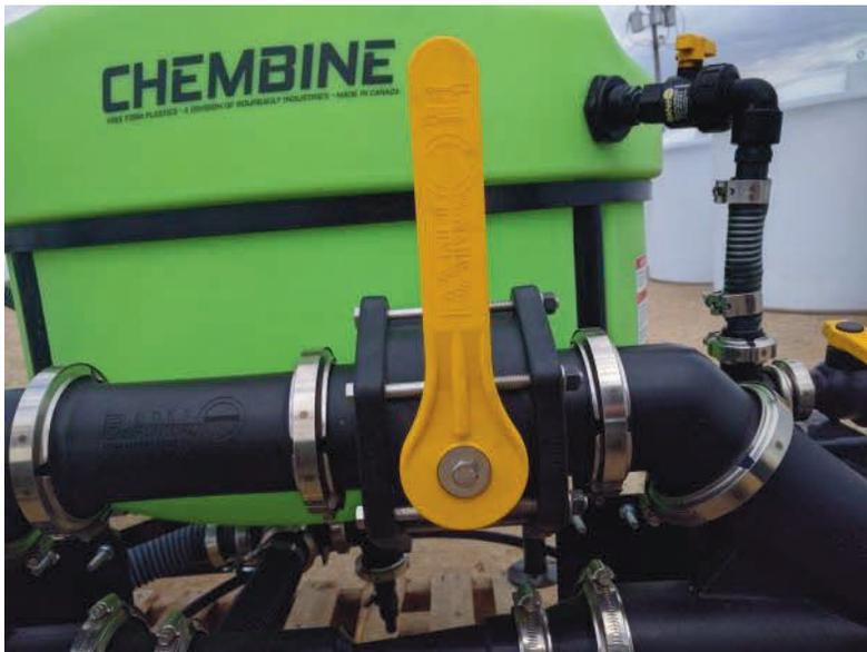
***Figure 2 - Bypass Valve Closed***
