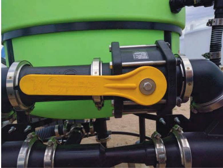
***Figure 1 - Bypass Valve Open***
