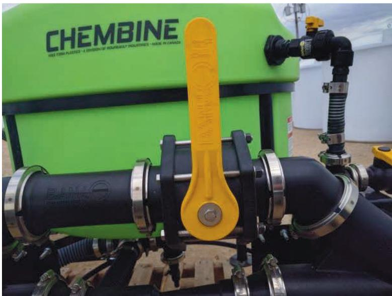
***Figure 2 - Bypass Valve Closed***
