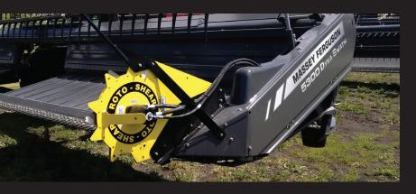
Each RotoShear kit comes complete with divider board, collector rod, mounting brackets and/or braces, hardware and hose kits as required. RotoShear's are available to fit almost all applications.
