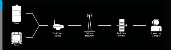
The Prophet 4000 Series, combined with TankData Online can help eliminate runouts and costly emergency deliveries, and increase operations efficiency up and down the supply chain. Using a standard internet browser, you can retrieve and use valuable tank information virtually anywhere in the world, whether the tank is local or a thousand miles away. You'll make smart, data-driven replenishment decisions, delivering more product left often, with fewer expensive truck rolls.
