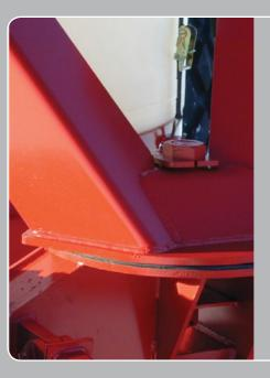
The front end of the Free Form LFC is engineered using the proven design of the Bourgault Air Seeder. This design allows for a full range of motion, along with outstanding durability. The large fifth wheel plate resists wear by utilizing a polymer wear pad. The front axle pivots on a lubricated pin and bushing system which offers rugged, trouble-free operation.
