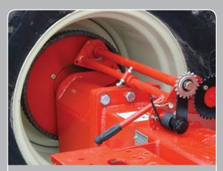
The mechanical ground drive system is "quick detach", has a spring loaded drive chain tensioner and features an adjustment bolt to allow the drive wheel chain and sprocket to remain tight.
