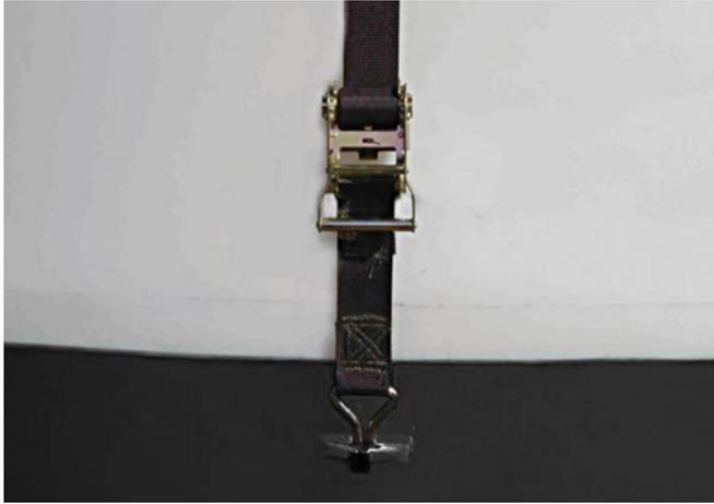
▶ Each tank is secured with three (3) custom-made straps. The straps are bolted to the lifting lugs on the top of the tank with 1/2" bolts and secured to the cone with ratcheting buckles. The ratcheting buckles allow for easy, and necessary adjustment to the strap tension, compensating for changing dimensions caused by temperature variations.
