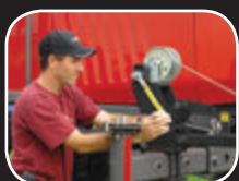
Adjustment is done manually with a winch/pulley system.
