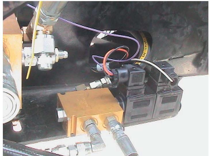
Figure 2.4 -Hydraulic Valve & fittings
