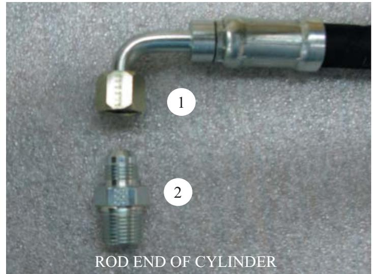
Figure 2.2 - Fitting Assembly of RIGHT Cylinder
