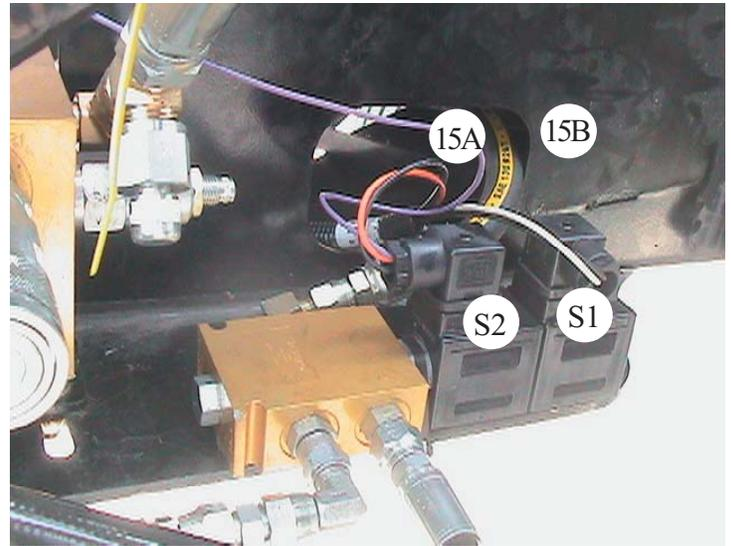
Figure 2.8 - Solenoid Connections
