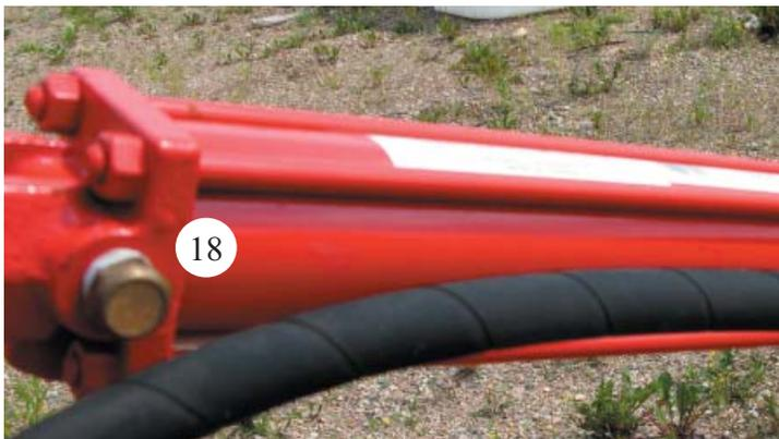
Figure 2.3 - Fitting Assembly of RIGHT Cylinder
