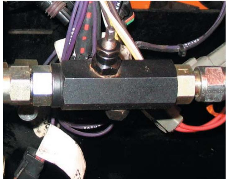
Figure 3.2 - Flow Control Valve
